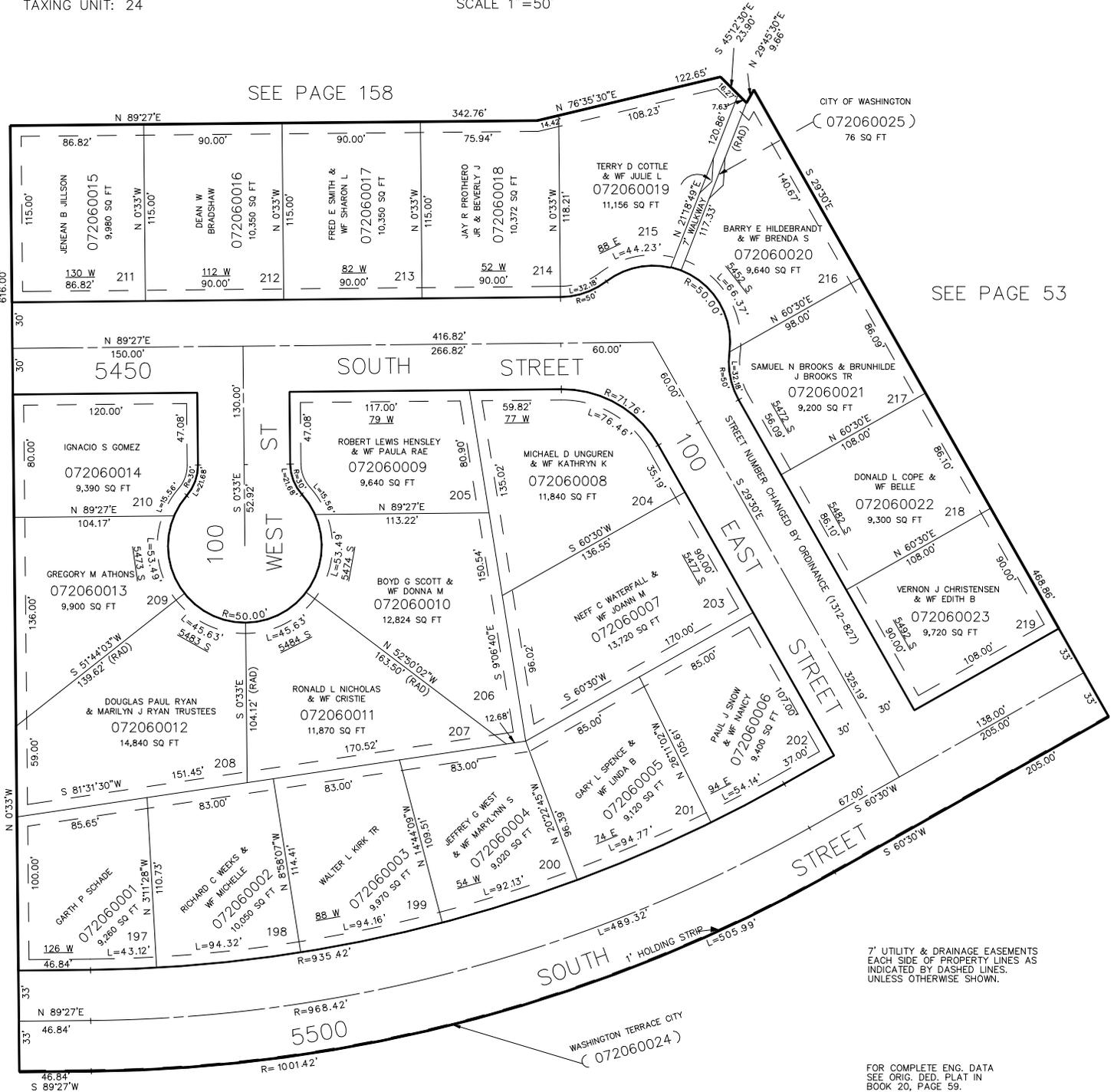
7' UTILITY & DRAINAGE EASEMENTS EACH SIDE OF PROPERTY LINES AS INDICATED BY DASHED LINES, UNLESS OTHERWISE SHOWN.
